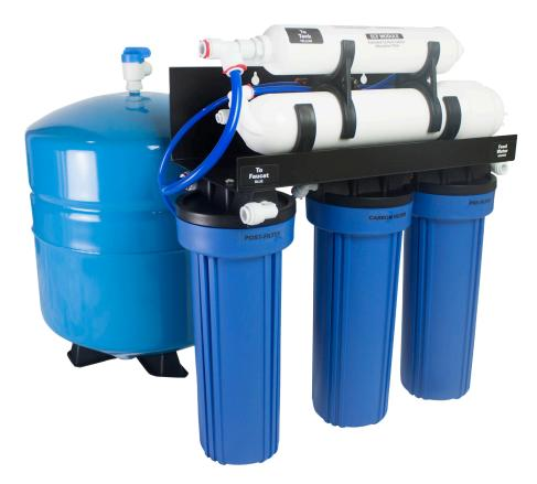
Self-contained 24-50gpd Reverse Osmoisis system, 5 micron pre filter, Extruded carbon block pre- filter, TFC membrane for rejection of dissolved solids, Nitrates, Salts etc. Post Carbon CTO block filter for taste (oxygenation) often you see the bubbles! Final prolonged contact VOC filter for extraction of MTBE, Benzene, Toluene, Atrazine etc...., Commercial/Industrial technology for the home or office!
